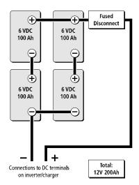
Figure 13 Batteries in Series-Parallel Connections
